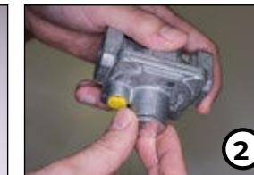
**2** - UN SCREW THE CAP TO ACCESS THE REGULATOR ADJUSTMENT.
